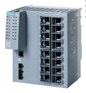
SCALANCE XC216 managed Layer 2 IE switch; IEC 62443-4-2 certified; 16x 10/100 Mbps RJ45 ports; 1x console port, diagnostics LED; redundant power supply; temp. range -40 °C to +70 °C; mounting: DIN rail/S7 mounting rail/wall Office redundancy functions features (RSTP, VLAN,...); PROFINET IO device; Ethernet/IP-compliant; C-plug slot;
