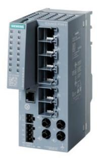
SCALANCE XC206-2 managed Layer 2 IE switch; IEC 62443-4-2 certified; 6x 100 Mbps RJ45 ports; 2x 100 Mbps ST/BFOC ports; 1x console port; diagnostics LED; redundant power supply; temp. range -40 °C to +70 °C; mounting: DIN rail/S7 mounting rail/wall redundancy functions; Office features (RSTP, VLAN,...); PROFINET IO device; Ethernet/IP-compliant C-plug slot;
