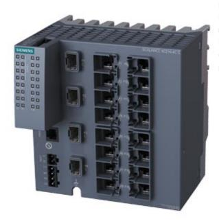
SCALANCE XC216-4C G managed Layer 2 IE switch; IEC 62443-4-2 certified; Full Gigabit; 12x 10/100/1000 Mbps RJ45 ports; 4x 1000 Mbps combo ports (either 1000 Mbps/ SFPs or 10/100/1000 Mbps RJ45 ports can be used); 1x console port; diagnostics LED; redundant power supply; temp. range -40 °C to +70 °C; mounting: DIN rail/S7 mounting rail/wall; redundancy functions; Office features (RSTP, VLAN,...); PROFINET IO device; Ethernet/IP-compliant; C-plug slot;
