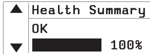
Figure 9: Residual-life indicator ("residual life")
