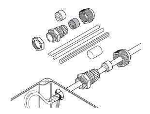
This connection kit is designed for terminating all nVent RAYCHEM BTV, QTVR, XTV, KTV and VPL industrial parallel heating cables to a junction box, whilst maintaining electrical insulation of the heating cable conductors and core.
