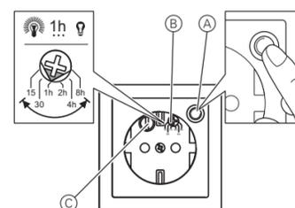
The timer socket-outlet can be switched off by pushing the button again before the time has elapsed. The timer socket-outlet has overload protection and short-circuit protection.
