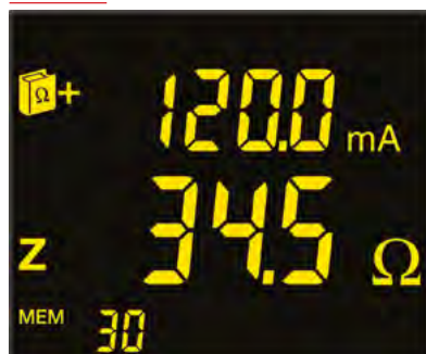
Screen 1: Impedance and leakage current
