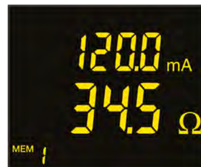
Standard mode: Impedance and leakage current
