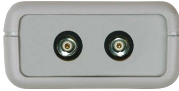
Simple Logger® II L102 Dual isolated BNC connectors accepts current probes with male BNC plugs
