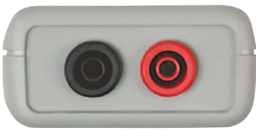
Simple Logger® II L261 Recessed safety 4 mm banana jacks
