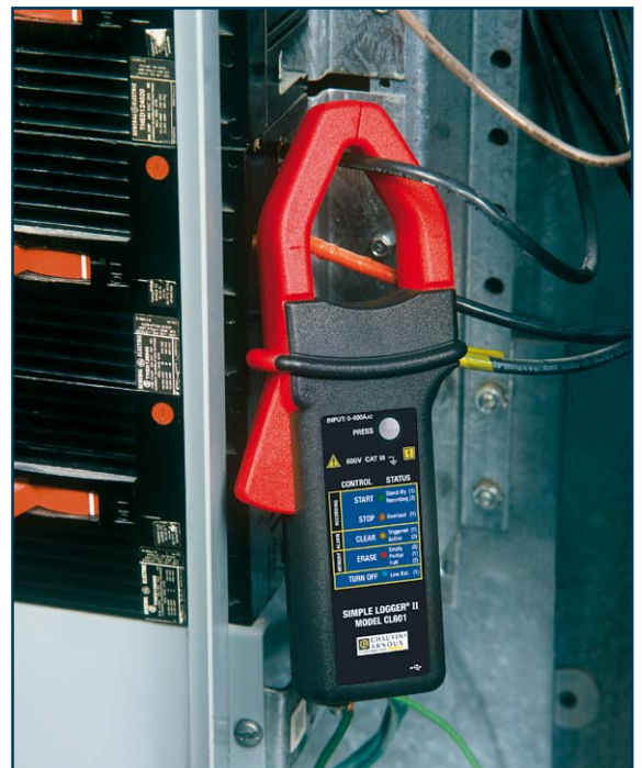
Easily log current in power panels.
