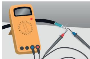
3. Check the insulation resistance of the heating cables. The measured value shall be no less than 50 MΩ.
