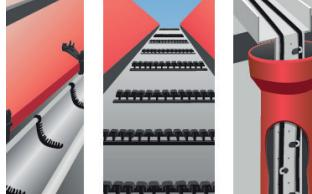
5. Install the connection box and fixing accessories in the gutters, gutter valleys, on the roof and/or the cable.
