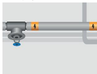
9. After insulation, place safety marking tape on the insulation jacket or pipe trenches for every 5 m. In subsurface installations, a cover ribbon with a warning sign must be laid 10 cm above the cables.
