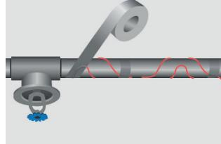
6. Apply aluminum tape below (mandatory for plastic pipes) and on top on the whole length of the cable. Make sure that the cables do not cross sharp edges.
