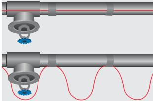
5. Straight lines and sensor must be fitted as shown at Fig.2. Twisted lines are attached as shown for every approx. 1 m pipe with aluminum tape.
