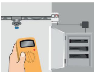
8. Re-check the insulation resistance. Connect cables to connection boxes and to the switch board.
