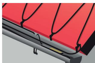
7. Install sensors and extend sensor cables, cold tails/terminate cables and place connections dry. Seal all penetrations, e.g. through roofs and walls.
