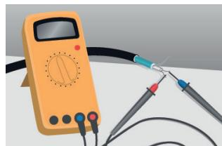
3. Verifique a resistência de isolamento dos cabos de aquecimento. O valor medido não deverá ser inferior a  $50\text{ M}\Omega$ .
