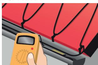
8. Check once again and compare the insulation resistance. The measured value shall be no less than 50 MΩ.
