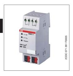
The diagnosis and protection module enables quick diagnostics of the bus state and indicates telegram traffic via an LED. A bus fault (U<U<sub>min</sub>) is indicated by normally open and normally closed contacts. The DSM incorporates a suppressor diode which suppresses transient overvoltages and interference voltage spikes on the EIB.
